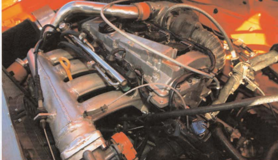
Thanks to a Garret T28 turbo and Weber Alpha management, this 1.8T unit is estimated to deliver around 300bhp. Nice!
