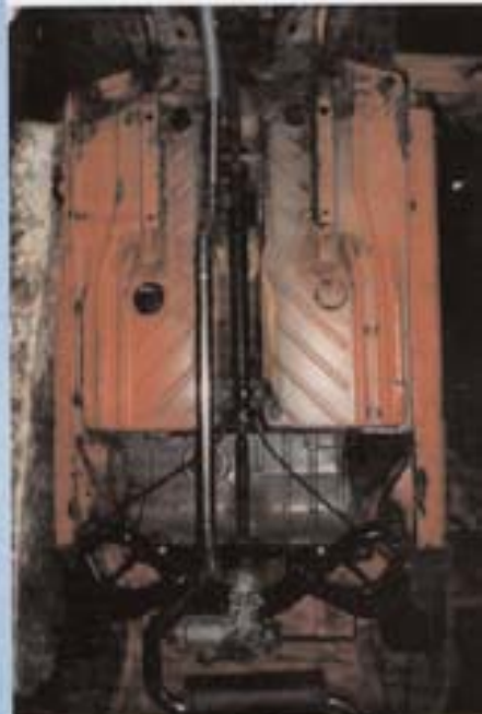
Detail of the shortened prop, custom exhaust and narrowed rear subframe
